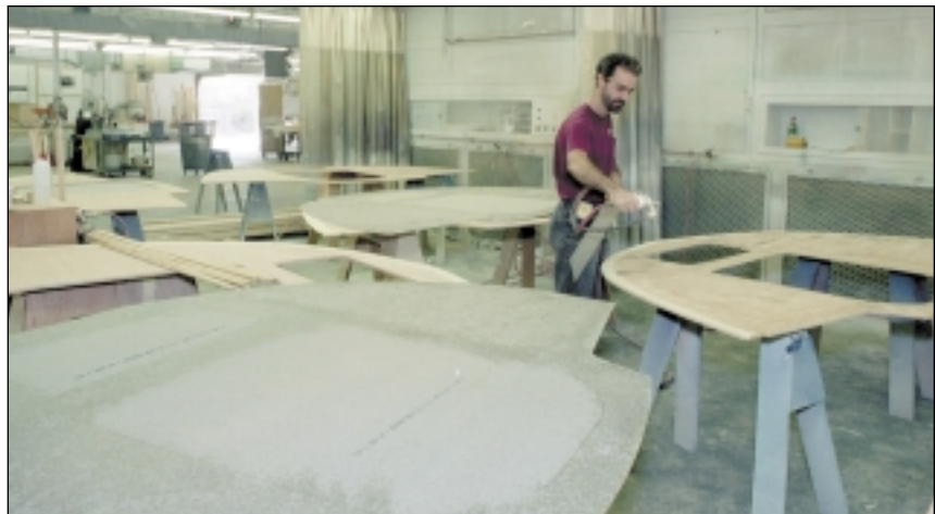
A large, fully air-filtered spray booth area is at the center of the 36,000-square-foot Jutras Woodworking facility. Here an employee sprays contact cement before laminating parts.
