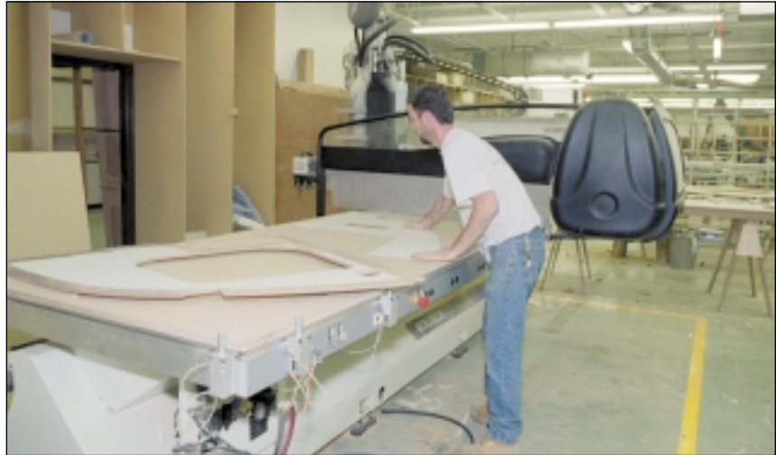
The SCM CNC router at Jutras Woodworking is used to machine many complex parts, often for boat interior projects. They also use the machine to make complex jigs and templates, and they even machine special forms like this one for better holding of complex parts for machining on the CNC itself.
