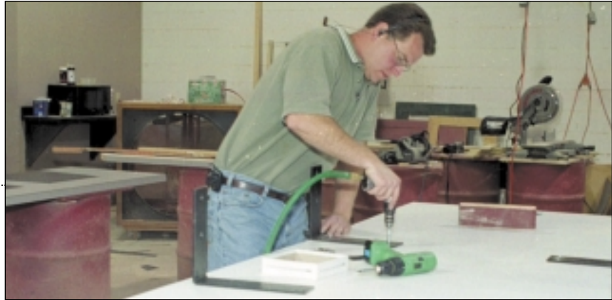
Screws and staples are the primary assembly devices for the work Atlanta Cabinet Shop does. Here an employee assembles a counterfront for a restaurant chain.
